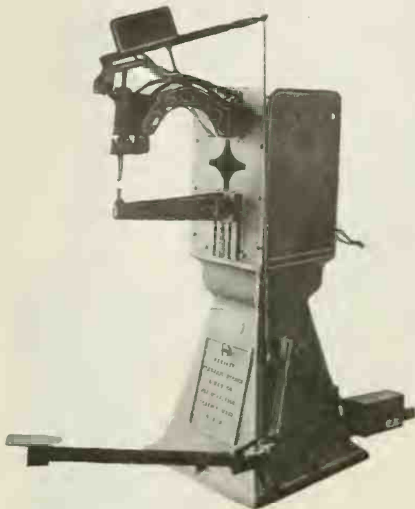
The Electric Spot Welder Here Shown Can Be Operated by Unskilled Labor and Does the Same Work As the Old-Fashioned Riveter, Faster and At a Much Lower Cost.
