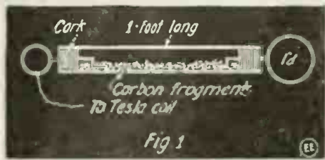
The High Frequency "Spark Tube"—It Comprises a Glass Tube Partially Filled with Powdered Carbon. It Is Charged by "Unipolar" Current from a Tesla Coil.
