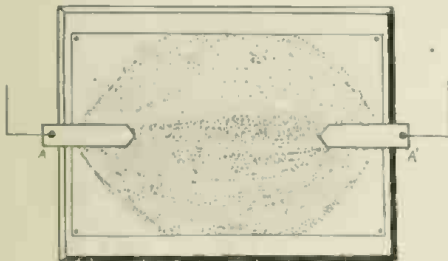
The Extent of a "Static Field" May Be Illustrated by Means of Fine Glass Particles (Powdered Glass) Spread on a Piece of Drawing Paper. A Small Static Machine Will Serve to Supply the Charge.
