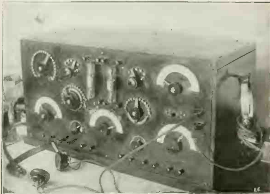
Appearance of Finished Damped and Undamped Valve Receptor. It is of the Cabinet Type and is Both Efficient and Attractive.
