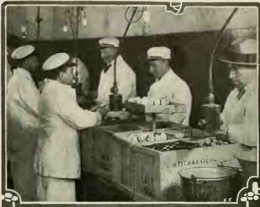
Here We See Nimble Fingred, Keen Eyed Egg Testers Separating the False from the True by Means of Electric Egg Candler, Operated from the Ordinary Lighting Circuit.
