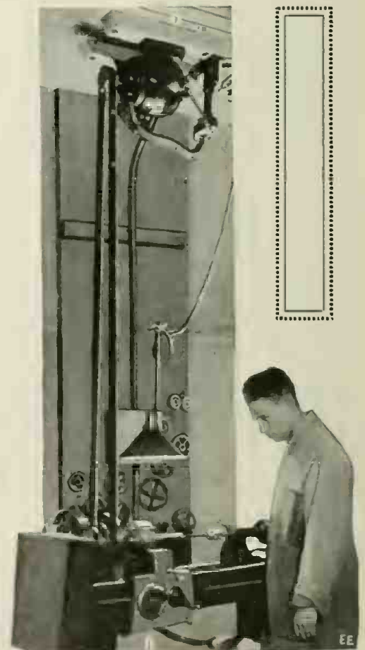
Fig. 4. A Good View of Actual Lathe Installation Equip With Motor Drive. A Drilling Operation Is Shown, the Drill Being Held in Tail Stock Chuck.
